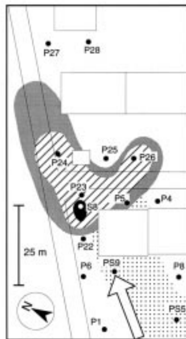
Figure 2b. Distribution of H 3 BO 3 94 days after the injection into PS9 (arrow). Sampled monitoring wells shown only.
